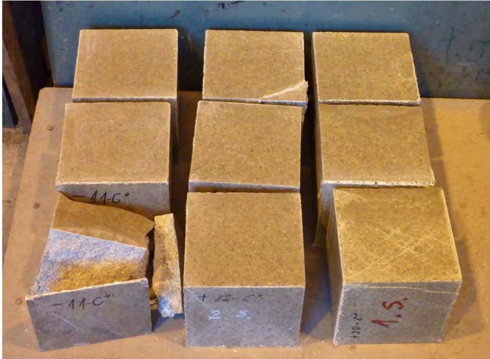
Fig. 1. Compression test specimens after failure
