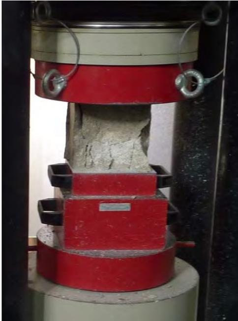
Fig. 3. *Compression test*
