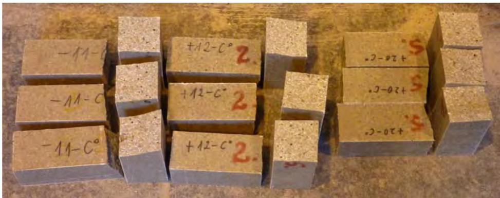
Fig. 2. Flexural test specimens after failure
