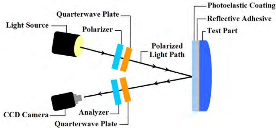
Fig.3. Simplified polariscope for photoelasticity by reflection
