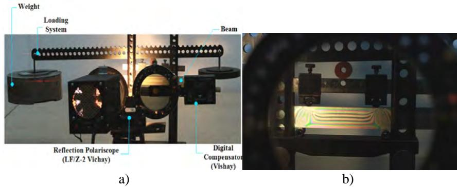
Fig. 4. a) The experimental set-up for calibration; b) Obtained fringes for beam with  $b = 2.6 \text{ mm}$
