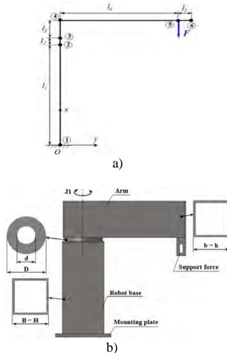
Fig. 1. a) The simplified scheme of the robot; b) CAD modeling
