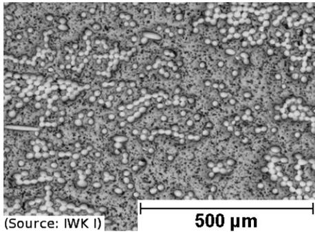
**Fig. 1:** Surface of polished LFT specimen
