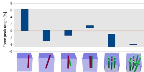
**Fig. 4:** Comparison of the peak force ranges for the examined cases of fibre topology (left to right) die slot distance, fibre inclination, two fibre models (orthogonal/parallel fibres), fibre clustering, random multifibre models.
