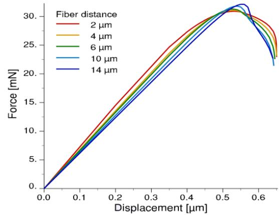
**Fig. 3:** Computed force-displacement-curves for the study of fibre density.
