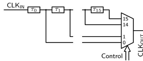
Fig. 1. The single digitally-controlled delay-element.
