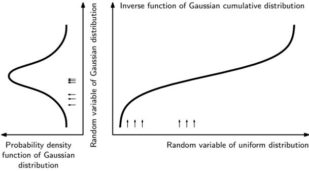
Fig. 4. The idea of obtaining random variable of Gaussian distribution.
