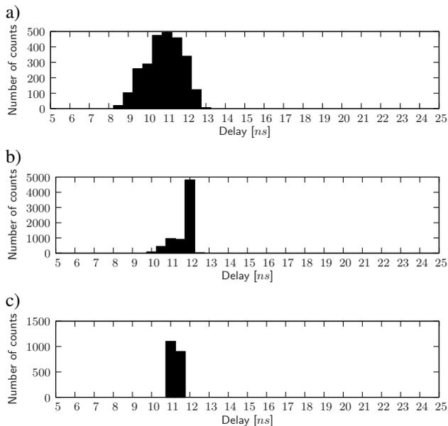
Fig. 17. Histograms of time-intervals of specified Gaussian distribution with constant average-value. Control-values change in ranges (a) (2,2,2,2,5,5,5,5), (b) (3,3,3,3,4,4,4,4) and (c) (3,3,3,4,3,4,4,4)
