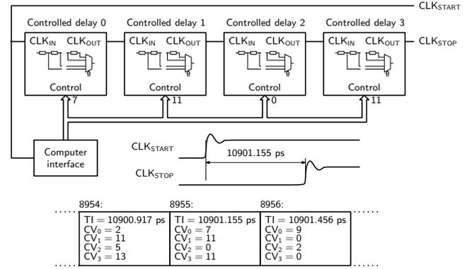
Fig. 5. Specified length time-interval generator.
