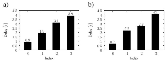
Fig. 2. The characteristic of the first (a) and the second (b) digitally-controlled-delay-element.
