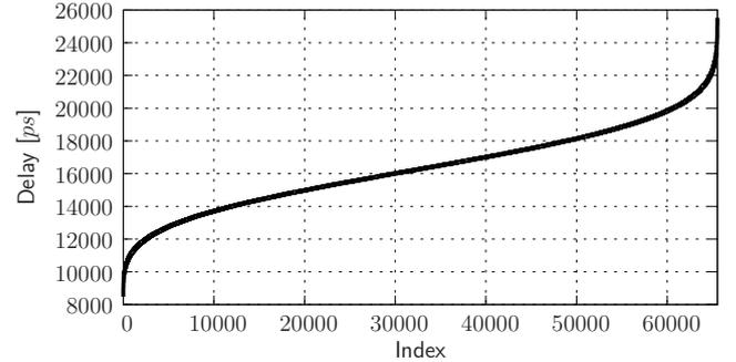
Fig. 9. DCDEs delay dependency from control-values index (control-values were changing in full range).
