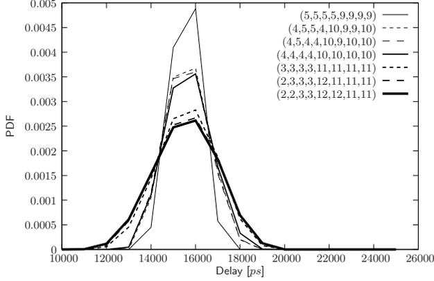
Fig. 14. Probability density functions of time-intervals obtained from serially connected digitally-controlled-delay-elements that characteristics have been presented in Fig. 12
