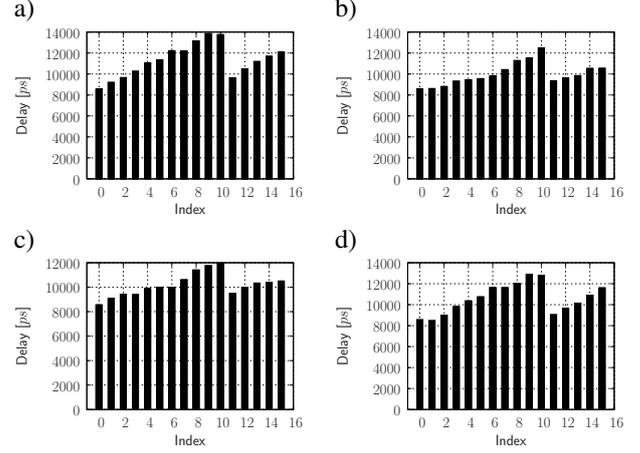
Fig. 8. The characteristic of the first (a), second (b), third (c) and fourth (d) digitally-controlled-delay-element.
