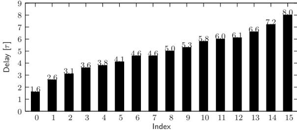
Fig. 3. The characteristic of two serially connected digitally-controlled-delay-elements.
