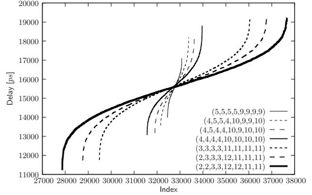
Fig. 12. DCDEs delay dependency from control-values. Control-values changes in such ranges that guarantee constant average-value and variable standard-deviation.
