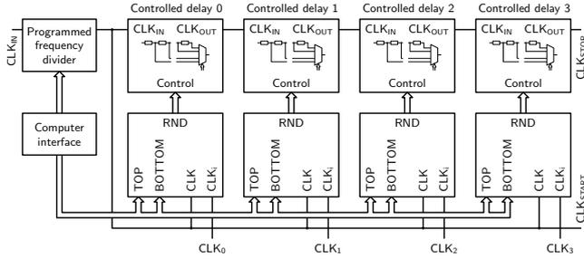
Fig. 7. Specified Gaussian distribution time-interval generator.
