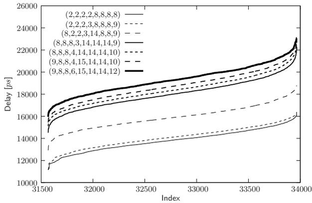
Fig. 11. DCDEs delay dependency from control-values. Control-values changes in such ranges that guarantee constant standard-deviation and variable average value.
