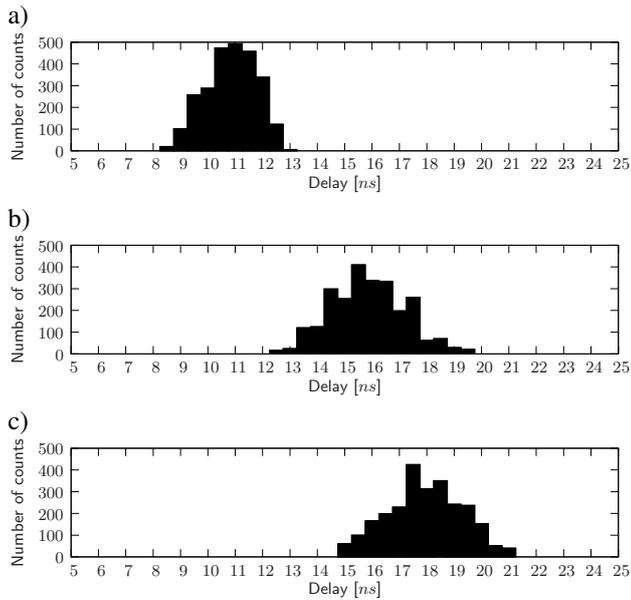
Fig. 16. Histograms of time-intervals of specified Gaussian distribution with constant standard-deviation. Control-values change in ranges (a) (2,2,2,2,5,5,5,5), (b) (5,5,5,5,8,8,8,8) and (c) (6,6,6,6,9,9,9,9)
