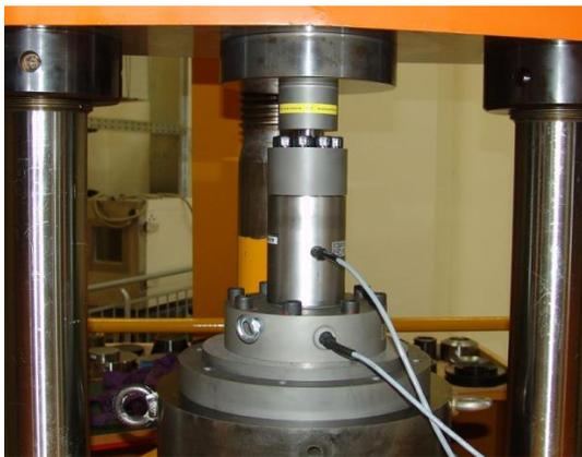
Fig. 3. Picture of the force calibration by using the 1-MN-FSM.
