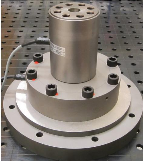
Fig. 2. Picture of the compression-torsion transducer.
