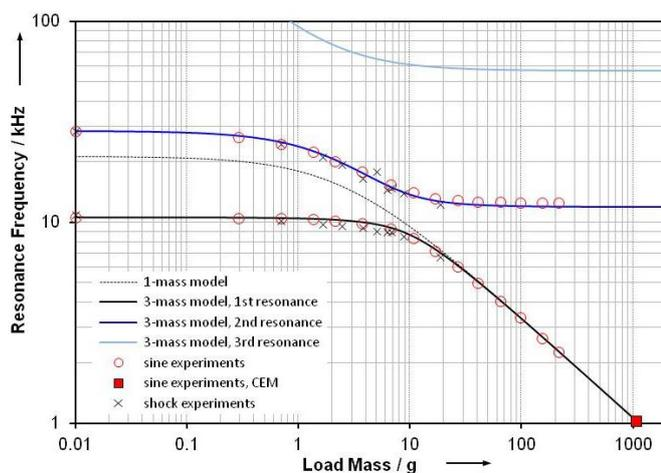
Fig. 12. Comparison of measured and modelled resonance frequencies of the HBM U9B / 1 kN with different load masses.
