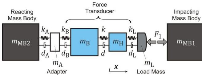
Fig. 8. Model of the 20 kN shock force calibration device with mounted force transducer and additional load mass.
