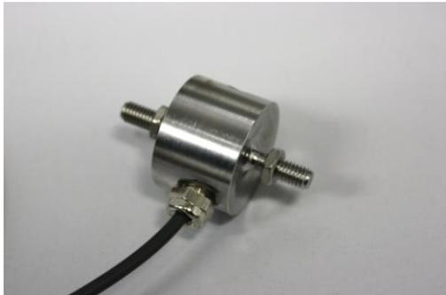
Fig. 1. Force transducer HBM U9B / 1 kN with a locknut at each bolt end.
