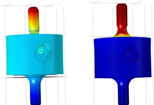
Fig. 2. FE simulation of the first two axial resonances of the force transducer HBM U9B / 1 kN fixed at the very end of the lower threaded bolt: colour-coded elongation of the transducer housing at the resonance frequency of 10.6 kHz (left), vibration of the head mass at 27.2 kHz (right).
