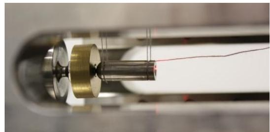
Fig. 4. Shock force tests at the 20 kN shock force calibration device using a pendulum of 7 g and an applied load mass.
