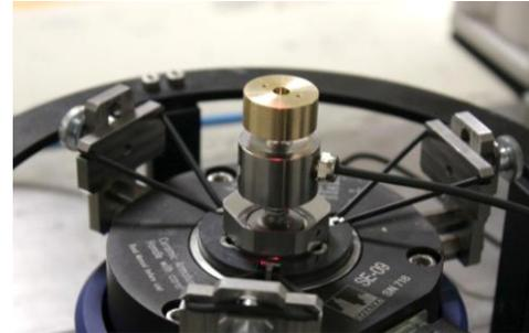
Fig. 6. High-frequency sine force tests with an additional load mass at the HF acceleration standard measuring device.
