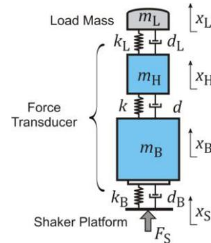
Fig. 10. Model of the sine force calibration device with mounted force transducer and additional load mass.
