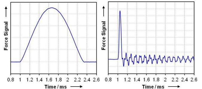
Fig. 3. Shock response of the force transducer HBM U9B / 1 kN using different impact masses, 10 kg (left), 7 g (right).
