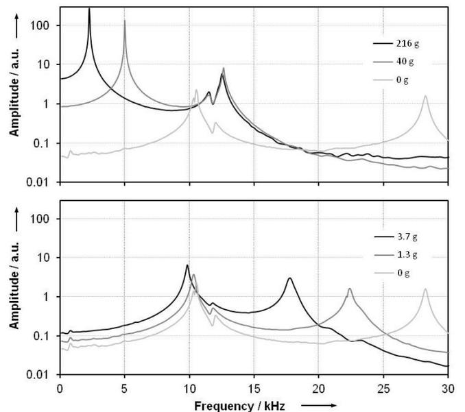
Fig. 7. Amplitude response (ratio of transducer output and base acceleration) of the HBM U9B / 1 kN obtained with different load masses measured at the HF acceleration standard measuring device.
