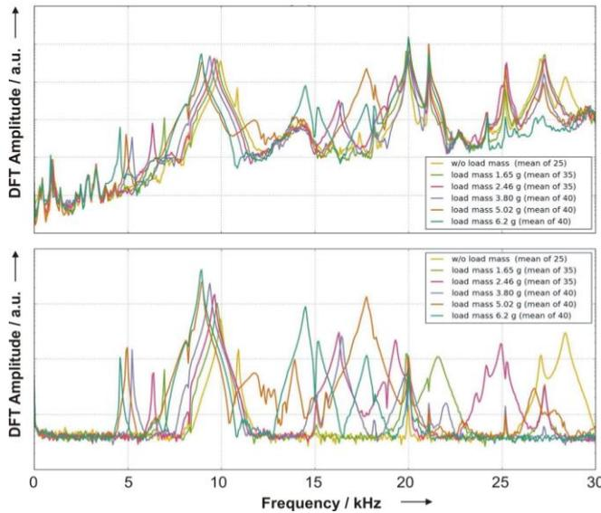
Fig. 5. DFT of the shock-excited ringing of acceleration  $a_2$  (top) and transducer output  $F$  (bottom) obtained with different additional load masses measured at the 20 kN shock force calibration device.
