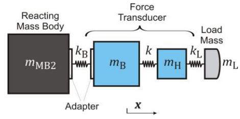
Fig. 9. Series arrangement of four model masses to describe the resonance frequencies of the 20 kN shock force calibration device.
