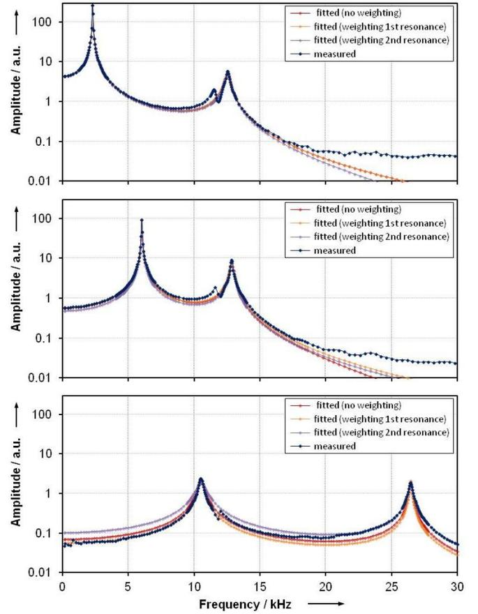
Fig. 11. Comparison of fitting procedures for the parameter identification from HF sine force measurements investigating the force transducer HBM U9B / 1 kN applied with different load masses of 216 g (top), 26 g (centre), and 0.3 g (bottom).
