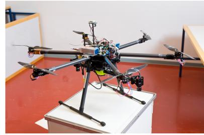
Fig. 6. MAV with the stereo camera system mounted in the bottom
