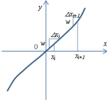
Fig. 1. Sample characteristics of FMM sensors;  $x$  – reading of a probe being calibrated;  $y$  – correct reading (real stylus displacement).
