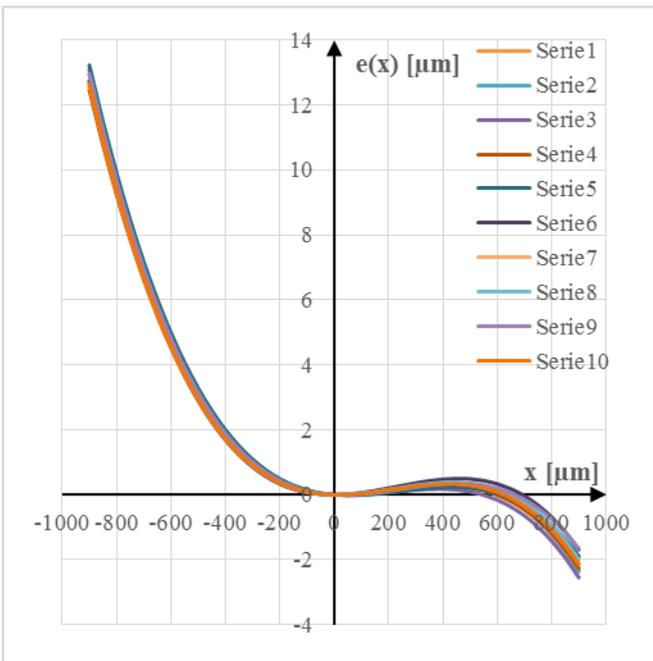
Fig. 7. Errors of Talymin 5 sensor characteristics obtained in 10 repetitions of the proposed procedure.
