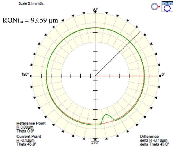
Fig. 3. Sample flick standard measurement result ( $x_i = 99 \mu\text{m}$ ).
