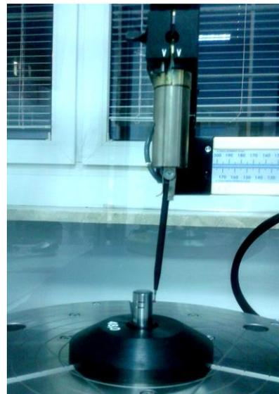
Fig. 2. Test stand – the Talyrond 365 and a flick standard on the table.
