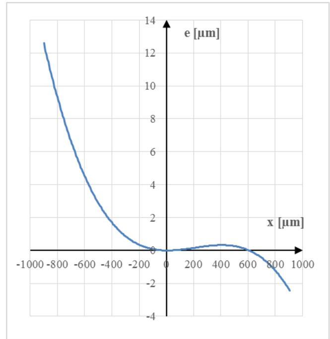
Fig. 5. Errors of Talymin 5 sensor characteristic obtained in the research.
