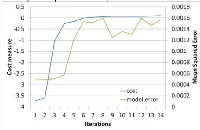
Fig. 6. Estimated cost of the optimum and model error over the iterations (normalized values)
