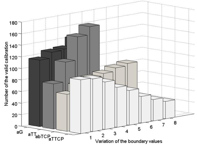
Figure 4: Variation of four boundary values and number of valid calibration with measurement noise, threshold value =  $50\mu\text{m}$
