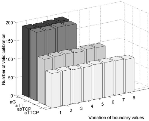
Figure 3: Variation of four boundary values and number of valid calibration without measurement noise, threshold value =  $50\mu\text{m}$
