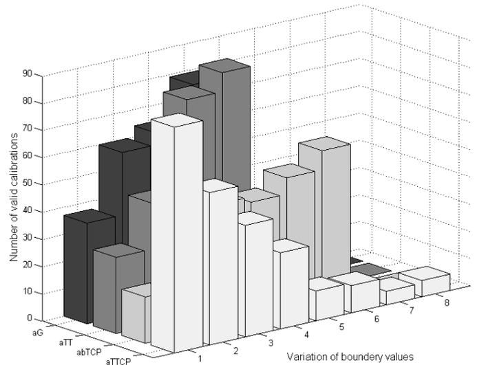
Figure 5: Variation of four boundary values and number of valid calibration with measurement noise, threshold value =  $10\mu\text{m}$
