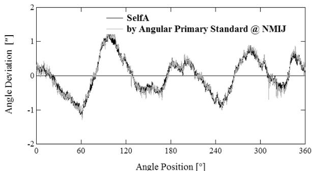
Fig. 6 The scale angular deviation analysis by SelfA and the angular primary standard at NMIJ.
