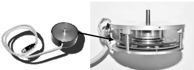
Fig. 4 The SelfA rotary encoder unit which built in the sensor heads circuit board and the scale disc.
