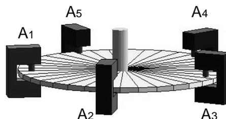
Fig. 1 Set up of self-calibratable rotary encoder. A1 is main head. ( $N_H = 5$  sensor heads).
