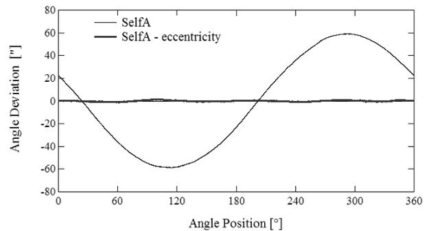
Fig. 5 Calibration result of SelfA rotary encoder.
