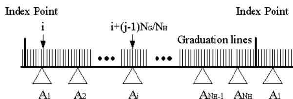
Fig. 2 Position relation between a rotary encoder scale and sensor heads of self-calibratable rotary encoder.
