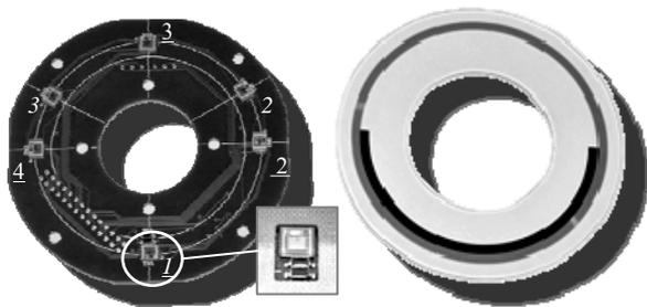
Fig. 3 The sensor heads array circuit board and its graduation scale for SelfA rotary encoder.
