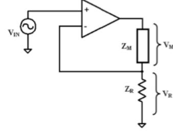
**Figure 2** Schematic for the transadmittance amplifier (voltage control current source)
