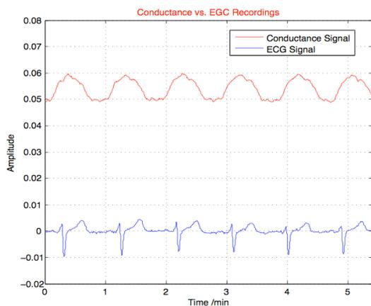
**Figure 4** Thoracic conductance recording obtained by the prototype with ECG synchronisation (aVR lead).
