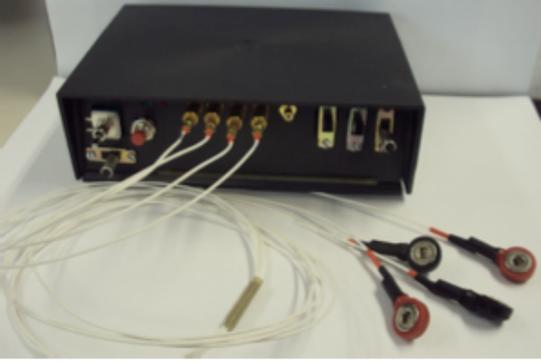
**Figure 1** Impedance measurement device developed. Capacitive electrodes were placed on an elastic belt.
