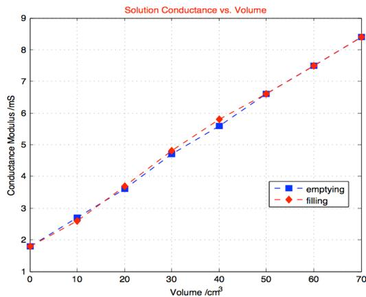
**Figure 3** Volume-related conductance measurements for filling and emptying with a  $0.141 \text{ Sm}^{-1}$  solution.
