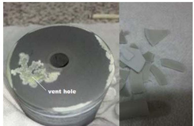
**Figure 4** Silicon vapour was found attached to the crucible around the ventilation hole (*left*) and the alumina discs become brittle after reaction with silicon vapour (*right*)
