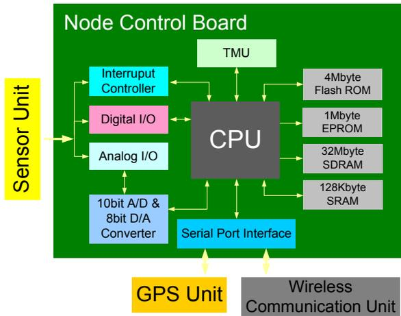
Fig. 3. System construction of sensing node.
