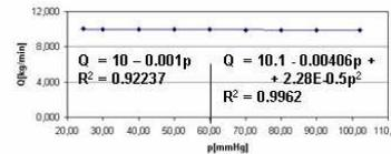
Fig. 3. Electrically controlled flow source FCFS
