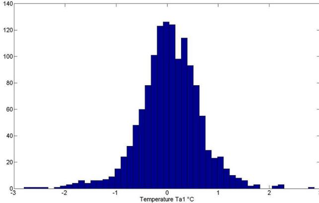
Fig. 5. Histogram of the standard deviations for the substitution error (for temperature  $T_{a1}$ ) for the mixture sensor  $M_{(Q,P,U)}$  providing the best performances in Table 1.
