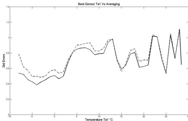
Fig. 3. Plot of the standard deviations of the substitution error (as subdivided for temperature) of the best trained soft sensor  $P$  (dash-dot line) among the 9 soft sensors used in the averaging procedure; plot of the average soft sensor  $P^{(9)}$  (solid line).
