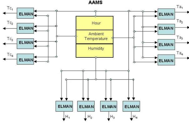
**Fig. 1. The connectionist system topology: twelve soft sensors of Elman type to measure contact temperature, humidity and air temperature in four locations of a monument (labels 1-4 correspond to the 4 locations).**
