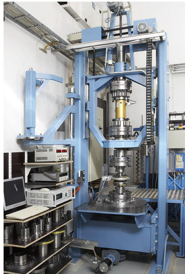
Figure 6 - View of the 20 kN·m torque reference device
