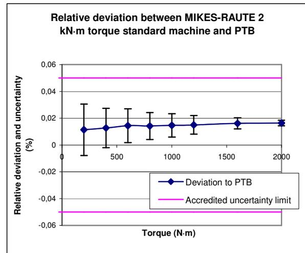
Figure 1 - Relative deviation and uncertainty of MIKES-RAUTE 2 kN·m torque standard device in comparison to PTB
