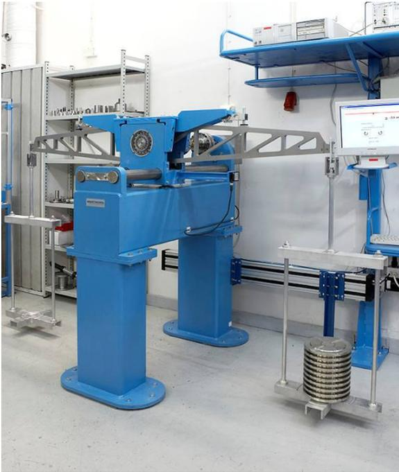
Figure 2 - View of the MIKES-RAUTE 2 kN·m torque standard device
