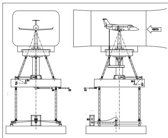
Fig. 2 - TA-2 external balance.  $R_1, \dots, R_6$  represent load cells.
