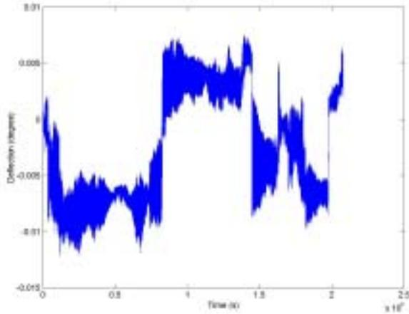
Fig. 5. Long holding modulated signal of photon pressure
