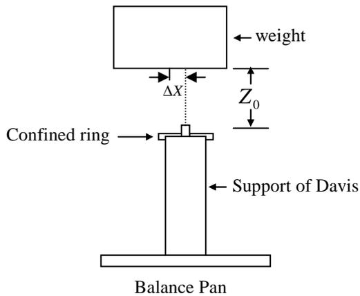
Fig. 2. Offset of the central line of the magnetic sample
