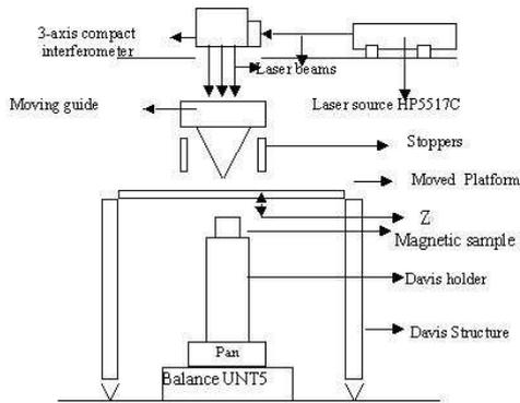
Fig. 1. Susceptometer in CMS
