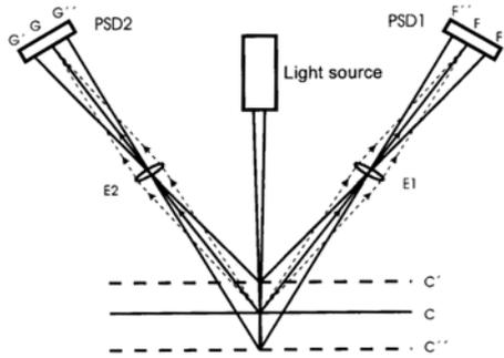
Fig. 2: Principle of triangulation
