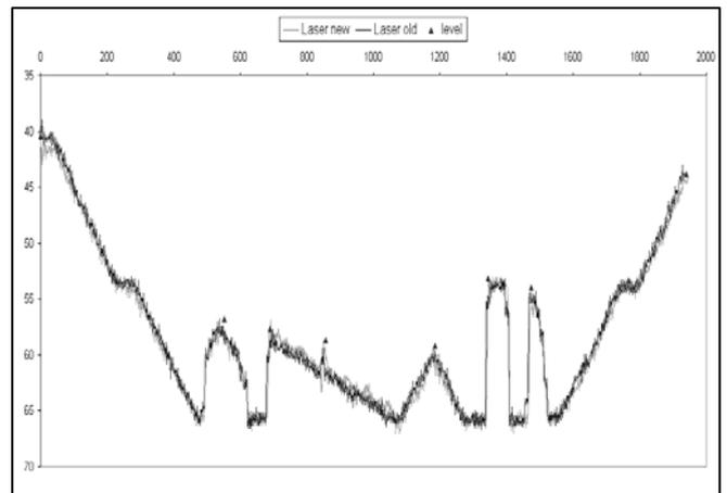
Fig. 5: Measured values of two laser-distance sensors compared with classically leveled values
