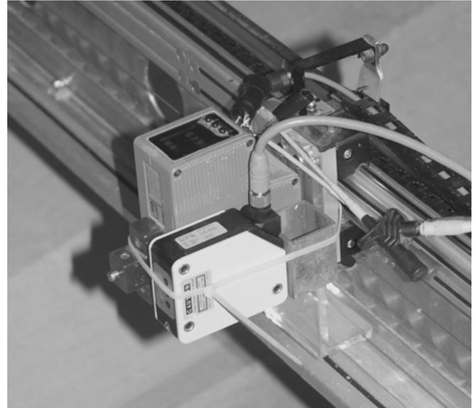
Fig. 3: Laser-based distance measurement instrument
