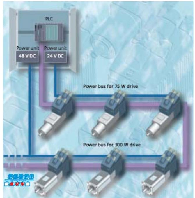
Fig. 8: Connection of POSMO A drive in control loop
