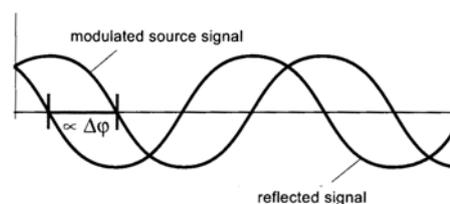
**Fig. 1: Principle of phase shift measurement**
