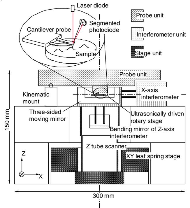
Fig.3. Nanometrological AFM<sup>[6]</sup>.
