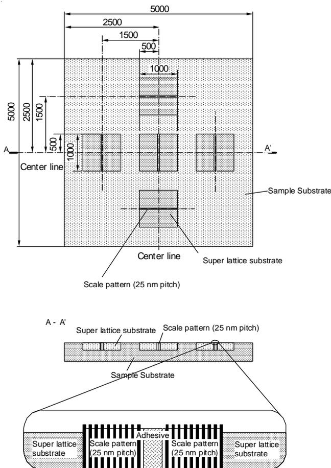
Fig. 2. Design of nanometric lateral scale.
