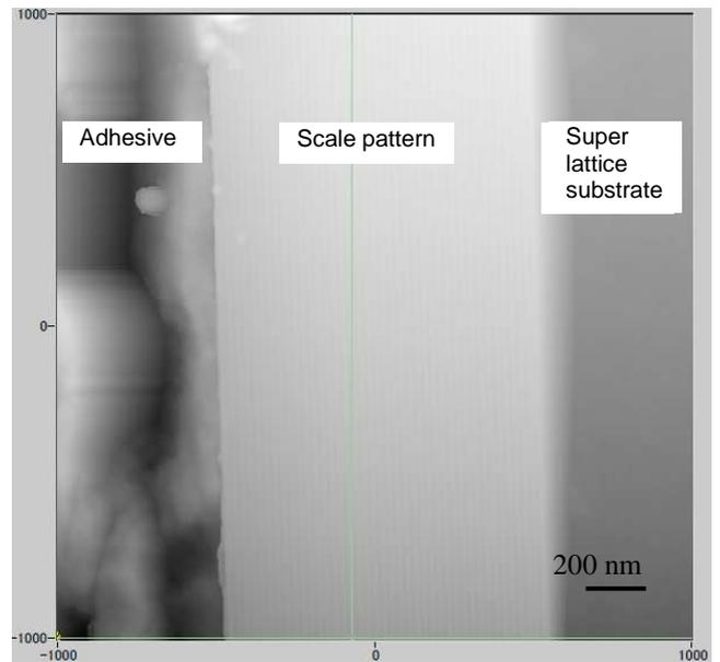
Fig.5. AFM image of nanometric lateral scale.
