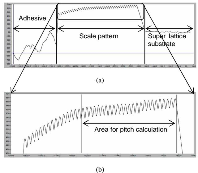
Fig.6. Area for pitch calculation.
