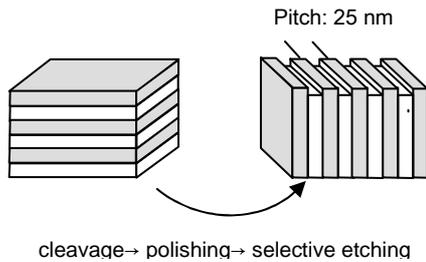
Fig. 1. Nanometric lateral scale consisting of superlattice.
