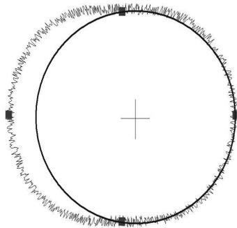
Fig. 2. Measurement of the circle with ovality deviation using 4 points
