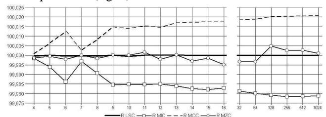
Fig. 4. The influence of the number of measuring points on the obtained radius of the measured circle for different fitting methods.  $MPE_E = \pm 2,5 \text{ [}\mu\text{m]}$
