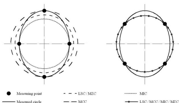
**Fig. 1. The results of roundness measurement influenced by the distribution of the measuring points and different fitting methods**
