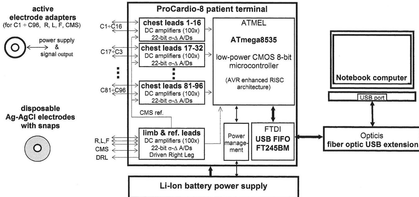
Fig. 1. Block scheme of the ProCardio-8 system
