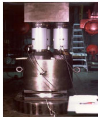
Figure 3. Setup for a 13 MN calibration.
