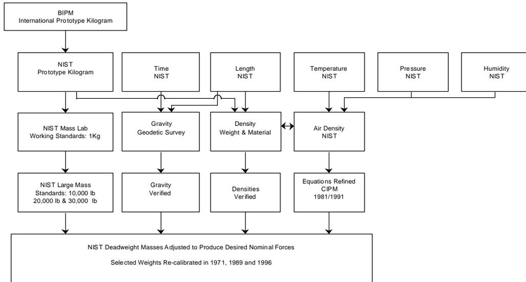
Figure 1. Traceability of NIST primary force standards to fundamental units.
