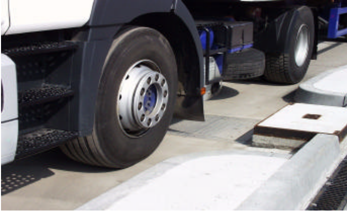
Figure 10. View of a truck crossing the weighbridge of an in-motion road vehicle weighing instrument ( Pfister )
