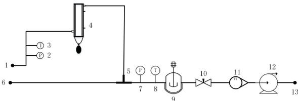
**Figure 3:** The electronic soap film flowmeter measurement part of flow standard device
