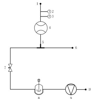
**Figure 4:** The roots flow-meter measurement part of the flow standard device
