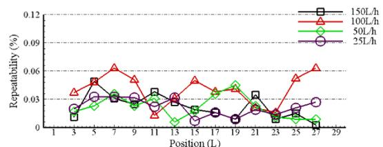
**Figure 2:** Device 2, the indication error (a) and repeatability (b) of different experimental sections of the piston cylinder at different flow rates with a verification volume of 2 L.
