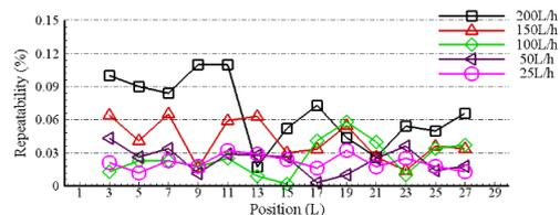
**Figure 1:** Device 1, the indication error (a) and repeatability (b) of different experimental sections of the piston cylinder at different flow rates with a verification volume of 2 L.
