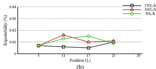
**Figure 6:** Device 2, the indication error (a) and repeatability (b) of different experimental sections of the piston cylinder at different flow rates with a verification volume of 6L.
