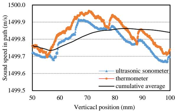
Figure 4: Sound velocity gradients in water tanks.
