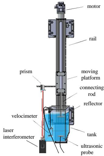
Figure 2: Schematic diagram of the experimental platform.
