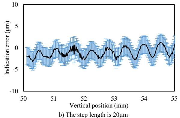
Figure 5: Schematic error of ultrasonic transit time difference measurement results.
