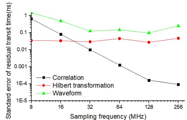
Figure 1: Response of the time difference algorithm to sampling rate.
