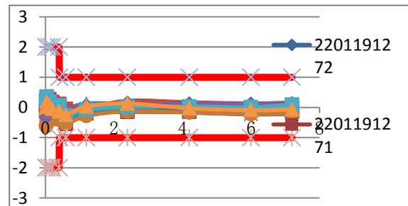
FIG. 8 Linearity measurement value of a batch of domestic gas flow sensor
