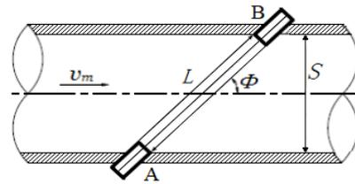
**Figure 1.** Schematic diagram of ultrasonic time difference method
