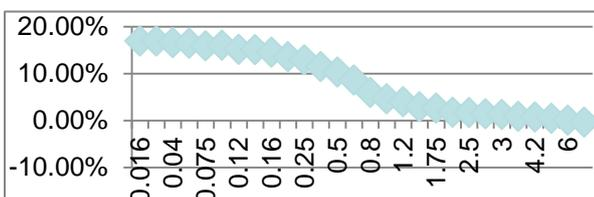
**FIG. 5** Correction factor between flow velocity profile and average velocity
