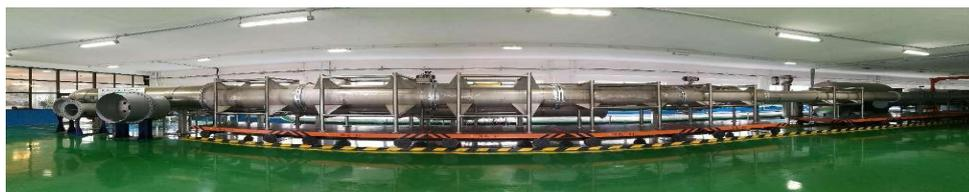
Figure 6. DN400~DN1200 positive looped dual-turbine standard meter method air flow rate standard facility
