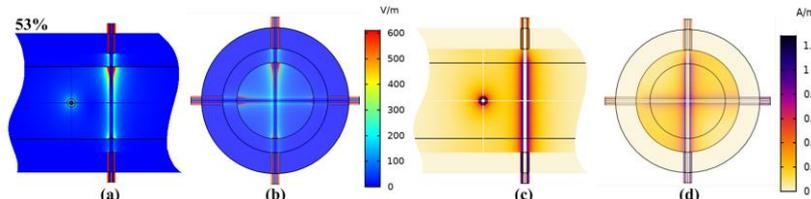
**Figure 3:** Electromagnetic field inside sensor (flow regime: annular distribution structure; void fraction: 53 %), where electric field intensity in front view (a) and in left view (b), magnetic field intensity in front view (c) and in left view (d).
