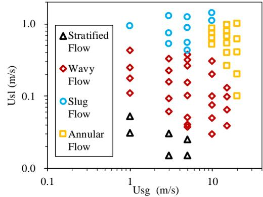
Figure 7: Flow regimes at different gas superficial velocity,  $U_{sg}$  and water superficial velocity,  $U_{sl}$ .
