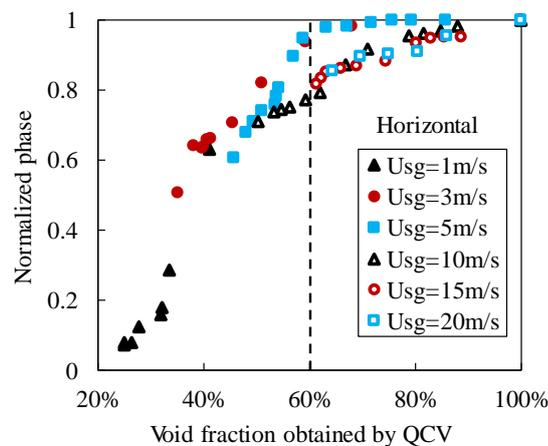
Figure 11: Relationship of  $P_{hor}$  and void fraction
