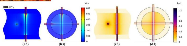
**Figure 2:** Electromagnetic field inside sensor (flow regime: stratified distribution structure; void fraction: 0 %, 53 %, 100 %), where electric field intensity in front view (a) and in left view (b), magnetic field intensity in front view (c) and in left view (d).
