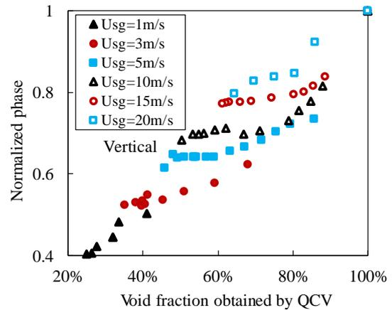
Figure 12: Relationship of  $P_{ver}$  and void fraction
