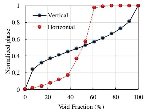
**Figure 5:** Relationship between normalized phase and void fraction.
