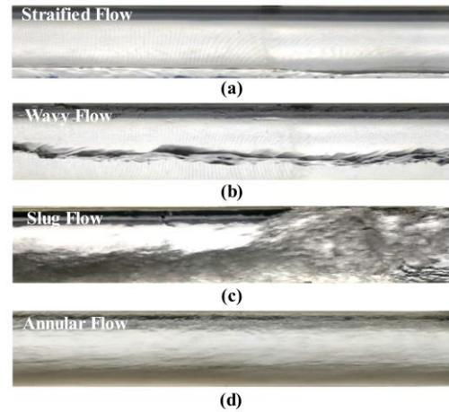
Figure 8: Pictures of flow regime (a) stratified flow at  $U_{sg} = 5\text{m/s}$  and  $\text{LVF} = 0.2\%$  (b) wavy flow at  $U_{sg} = 5\text{m/s}$  and  $\text{LVF} = 0.8\%$  (c) slug flow at  $U_{sg} = 10\text{m/s}$  and  $\text{LVF} = 5\%$  (d) annular flow at  $U_{sg} = 20\text{m/s}$  and  $\text{LVF} = 3\%$
