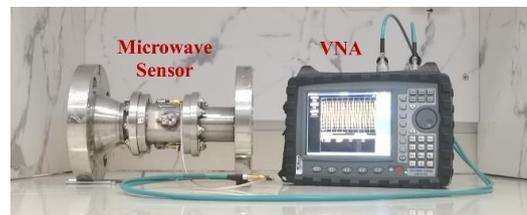
**Figure 4:** Static measurement system.
