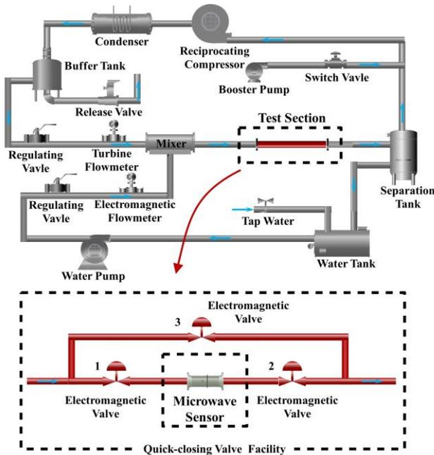
Figure 6: Sketch of wet gas flow facility [11, 12] and quick-closing valve facility.
