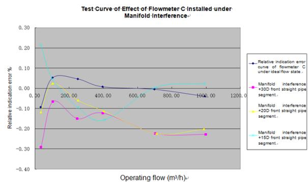
According to the above figure: ① Under the condition of manifold interference, the relative indication error curve trends of flowmeter C in the ideal flow state and at 30D and 20D of the upstream straight pipe segment are basically the same. The maximum change is not more than 0.21%. ②The relative error curve has different trends at 15D of the upstream straight pipe segment, with the maximum change up to 0.32%. ③Under manifold interference, when the operating
