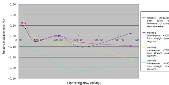
According to the above figure: ① Under the condition of manifold interference, the relative indication error curve trends of flowmeter D in the ideal flow state and at 30D and 20D of the upstream straight pipe segment are basically the same. The maximum change is not more than 0.23%. ②The relative errors of the upstream 15D straight pipe segment are obviously different. The FLOMEKO 2022, Chongqing, China
