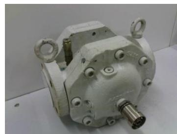
Figure 1 – Rotary gas meter Actaris Delta S-Flow
