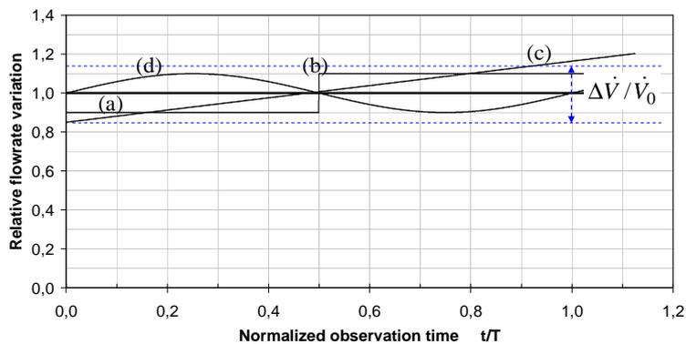
**Figure 5** Calibration facility: flowrate time characteristics
