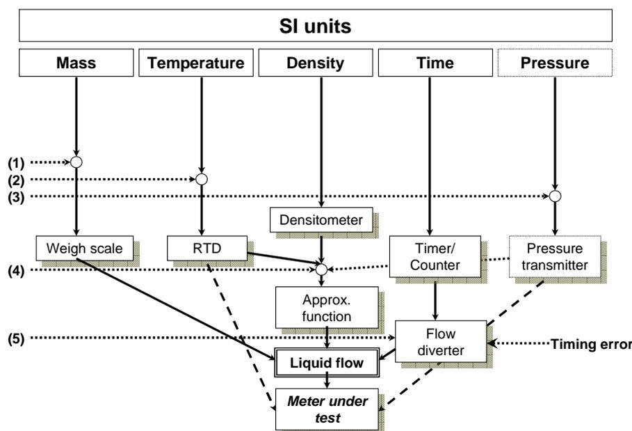
**Figure 2** “Comprehensive” traceability chain in fluid flow calibration - comprising dynamic process effects on the measurement uncertainty of liquid-flow standard facilities:
