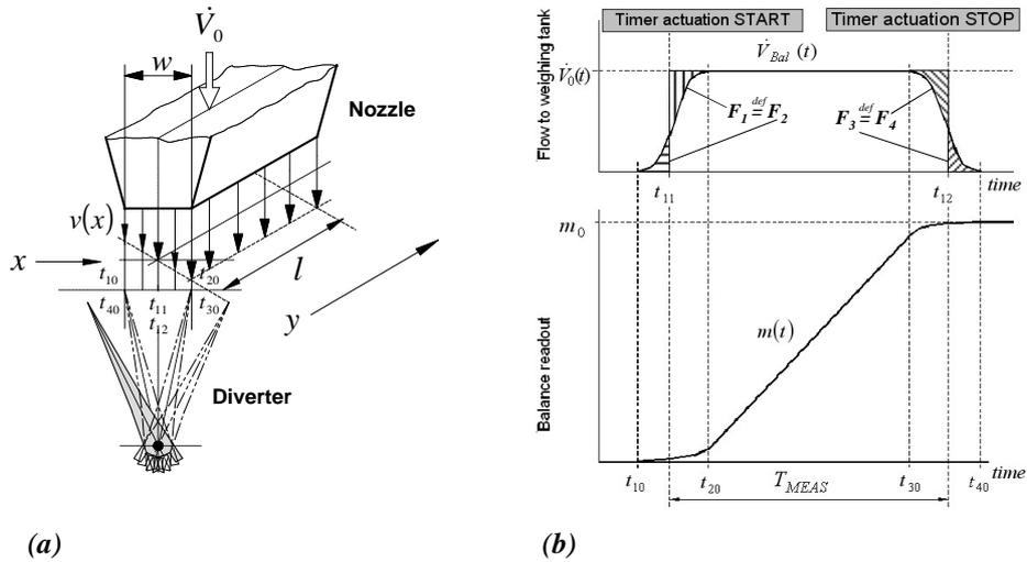
**Figure 4** Principle of flow diversion
