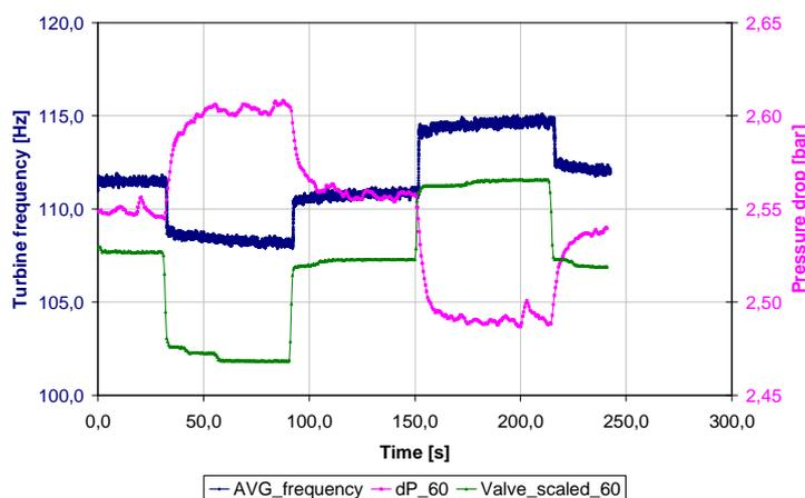
**Figure 8** System reactions upon step-like variations of control valve position:
