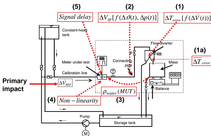
**Figure 1** Gravimetric liquid flow calibration facility – Uncertainty impacting items and impact of flowrate fluctuations
