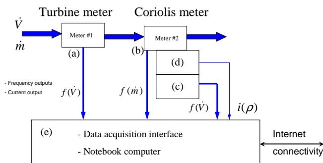
Figure 6 Calibration facility: monitoring the flowrate time characteristics - auxiliary electronics for monitoring the dynamics of process flowrate
