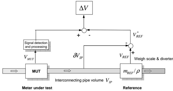
**Figure 3** Main elements of flow calibration facilities
