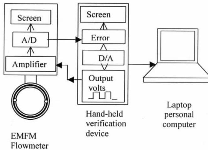
Figure 2 Typical set-up for verification tool, EMFM and computer
