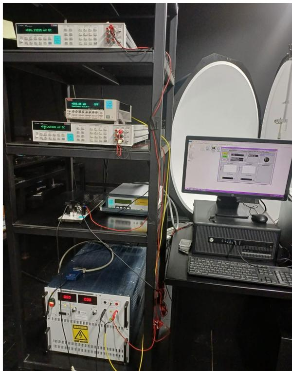
Fig 3. Photometric Measurement Equipment
