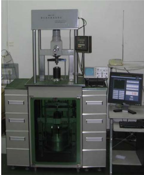
Figure 6 the picture of the new Rockwell hardness primary standard machine
