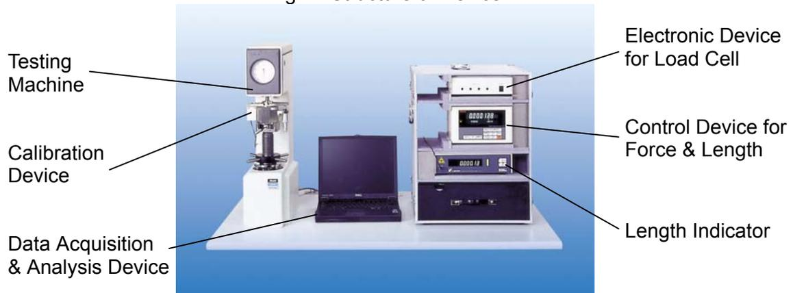
Fig. 2 Device installed on H. Tester
