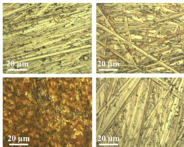
**Fig. 4.** Micrographs of the quaternary 555 alloy disks with a high roughness before (first row) and after (second row) corrosion treatments with HCl/H<sub>2</sub>O vapours for bare alloy (on the left) and coated with chitosan-BTA (on the right).
