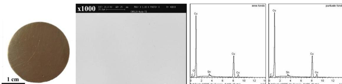
**Figure 2.** Photograph, SEM image and EDS spectra of bare CNR- alloy. The EDS spectrum on the left was recorded on a large area and the one on the right on the white islands.
