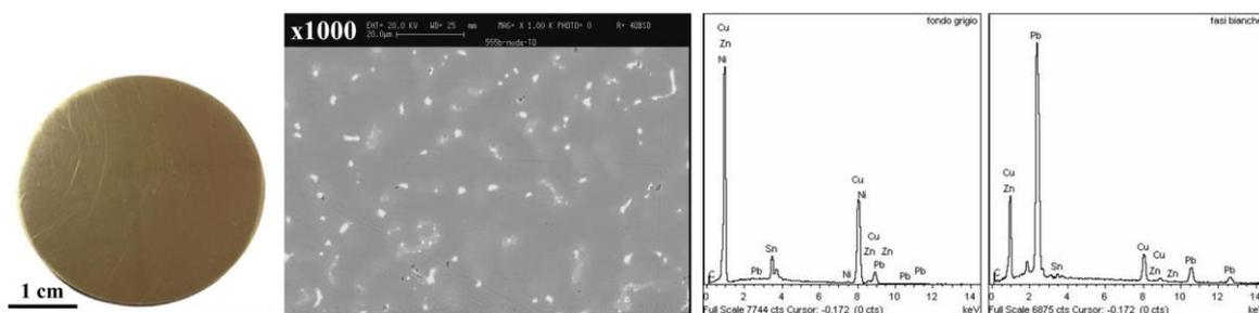
**Figure 1.** Photograph, SEM image and EDS spectra of bare 555 alloy. The EDS spectrum on the left was recorded on a large area and the one on the right on the white islands.
