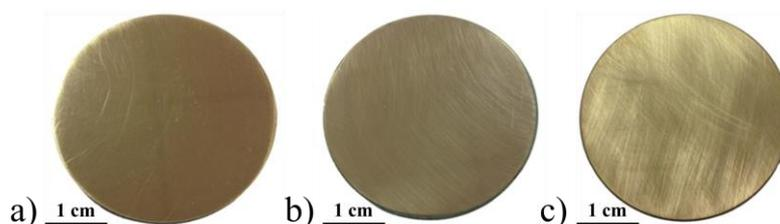
**Fig. 3.** Photographs of alloy disks with different surface roughness: a) 555-SF1, b) 555-SF2 and c) 555-SF3.
