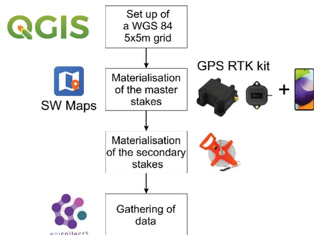
Figure 1. Gathering the data: software and hardware
