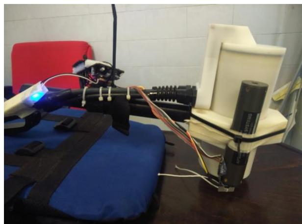
Fig. 3. The testing set-up with the GEM-19 magnetometer and the prototype.
