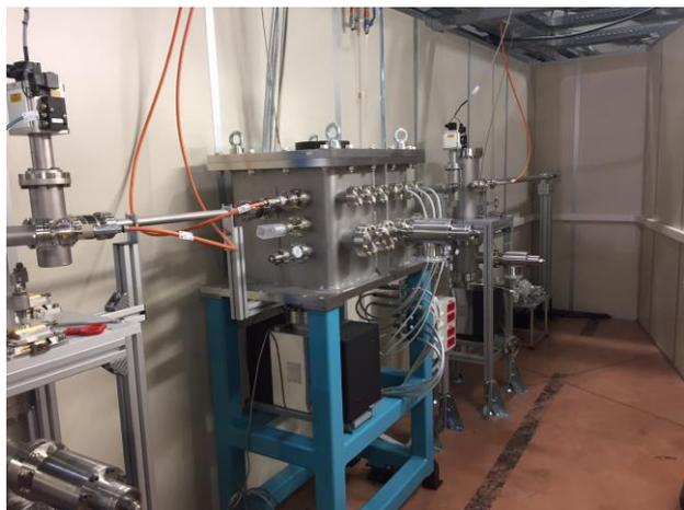
Fig. 9. The XRF monochromator
