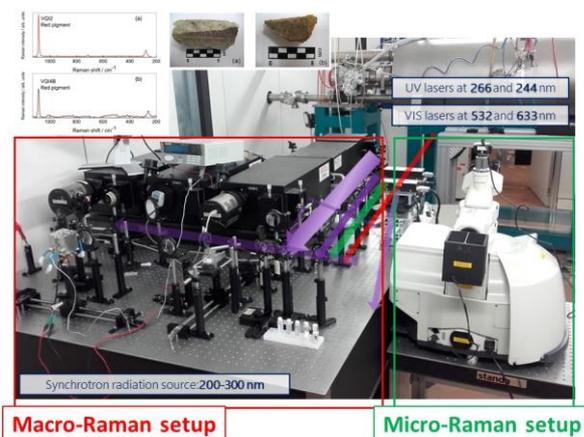
Fig. 3. experimental setup for macro- and micro- UV Resonant Raman spectroscopy measurements at IUVS. The exciting radiation source is provided by synchrotron radiation and by conventional laser sources in the UV and visible range.
