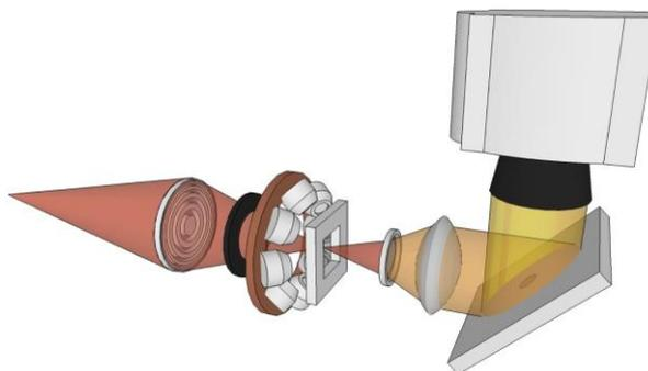
Fig. 8. Scheme of the TwinMic final stage. On the left a zone plate forms a microprobe which is sent to the specimen on a scanning stage for XRF analysis. On the right a configured transmission detector system with visible light converter.
