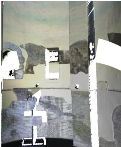
Fig. 3: A screenshot of RGB-ITR laser coloured mesh of the room. This preliminary result is obtained just by applying the calibration dataset to the raw laser scanner data
