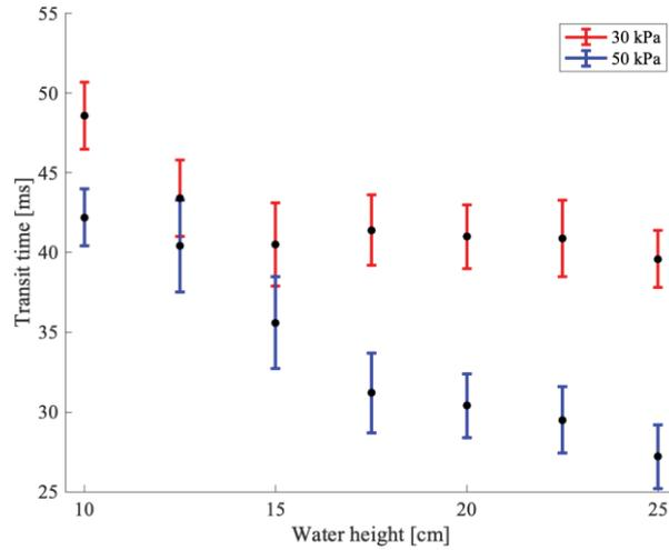
Fig. 3. Transit time and water height relationship with error bars due to standard uncertainties.
