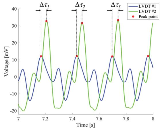
Fig. 2. Differences between the peak time instants of the two LVDT waveforms for inner pressure  $p_i = 50$  kPa.
