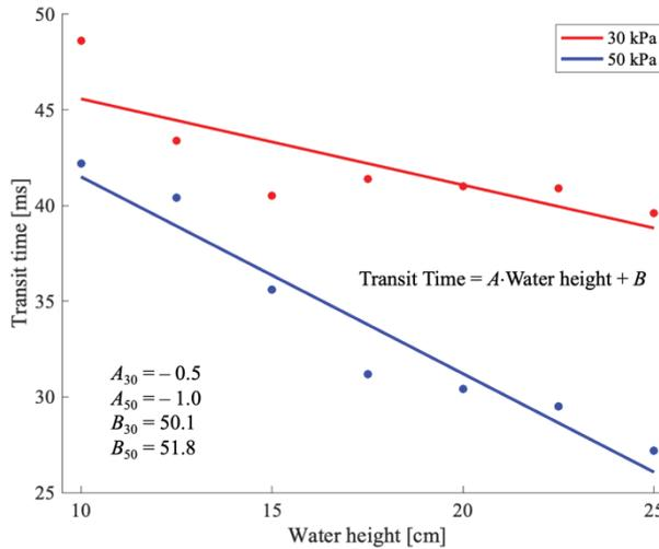
Fig. 4. Least squares method applied to the mean transit time values for increasing outer pressure.
