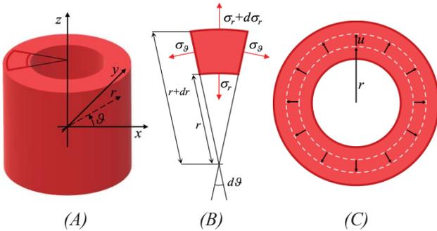
Fig. 1. (A) Cylindrical coordinates system; (B) Equilibrium of the element of volume in the plane  $r$ - $\theta$ ; (C) Static radial displacements  $u$ .
