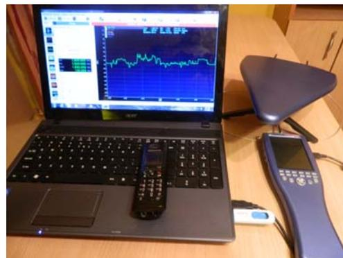
*Fig. 1. Radiofrequency measurement set-up, based on Spectrum Analyzer SPECTRAN HF 60105 Hyper LOG 60100 antenna and MCS dedicated AAronia software*
