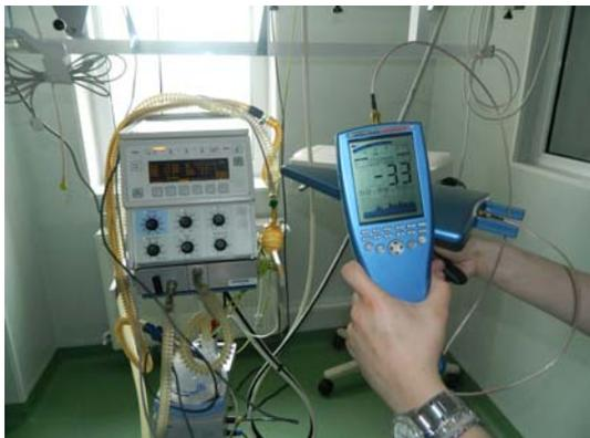
*Fig. 2. Measuring the EM environment of Drager Babylog 8000 neonatal ventilator*
