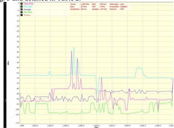
Fig. 3. Display of the DECT spectrum
