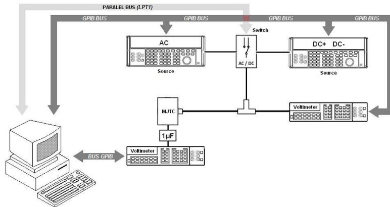
Figure 1: PMJTC Measurement system using Swerlein algorithm
