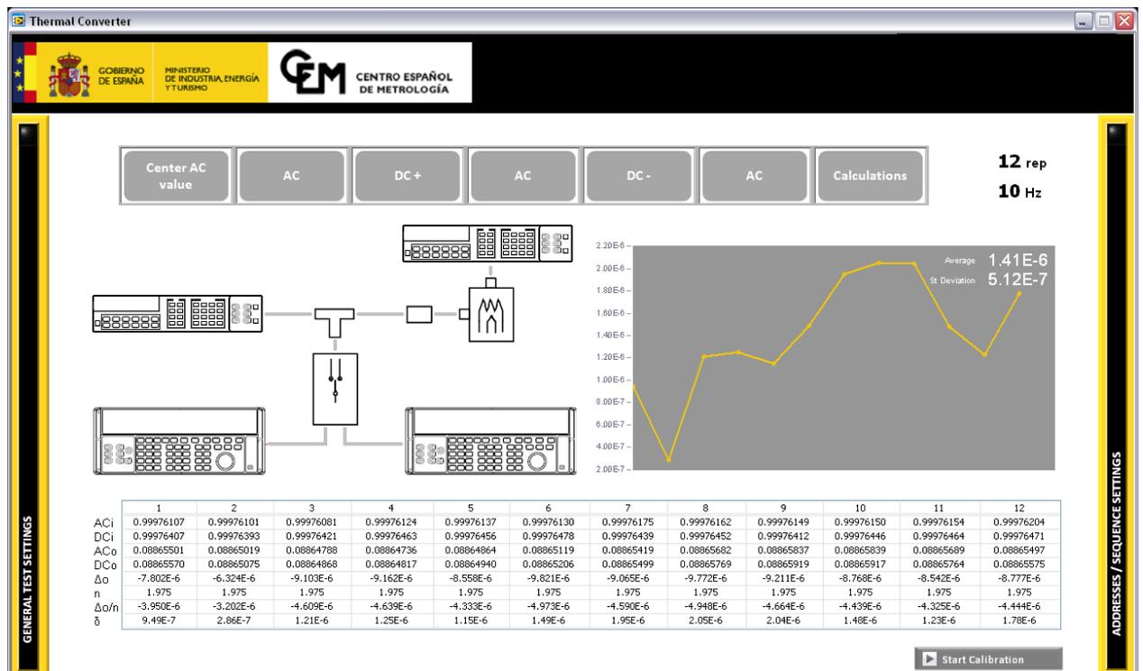
Figure 2: Front panel of the software used for the characterization of ac-dc transfer difference
