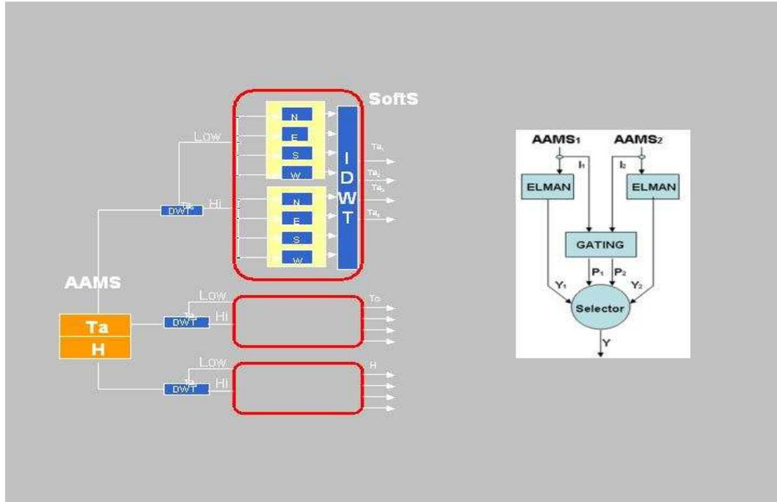
Fig. 1. (Left) The connectionist system topology with the wavelet decomposition (completely displayed only for air temperature parameter): twelve soft sensors of Elman type are used to simulate  $T_a$ ,  $T_c$  and humidity  $H$  in four locations, with and post wavelet processing. (Right) The mixture of two local experts whose input sources are two AAMS, with a gating NN.
