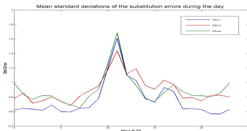
Fig. 2. Plots of the standard deviations of the substitution error (as subdivided for hour) for air temperature: simple Elamn soft sensor (green line); with wavelet preprocessing Db2 at level 1 (blue line); Db2 at level 2 (red line).
