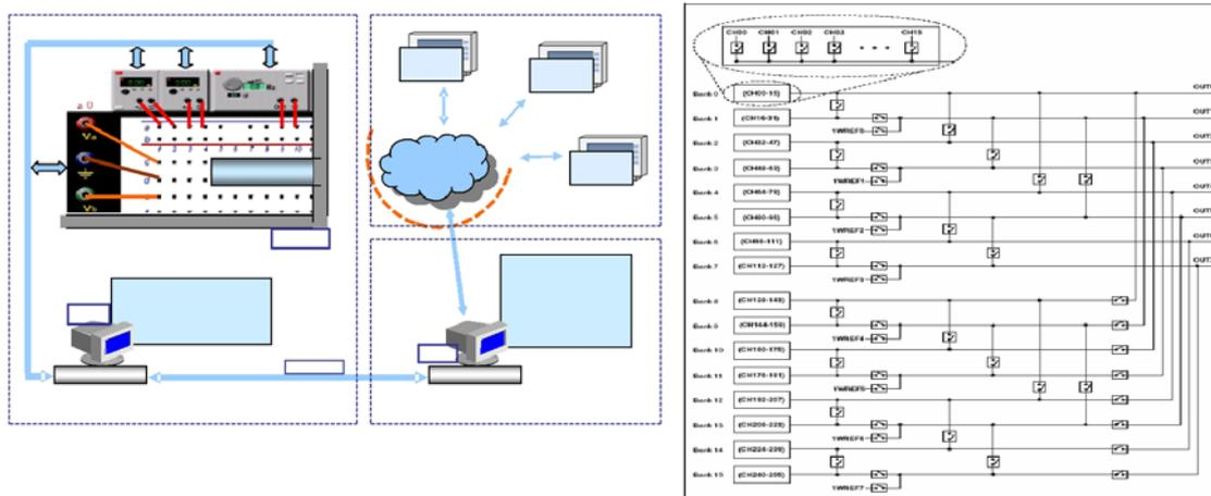
System's architecture (figure 1) is structured on three main levels: reconfigurable workstation level, multitask server level and user server. Initiating the execution of a laboratory work comes from the user level, by accessing the server's web interface through a commercial browser.
