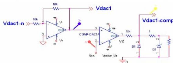
Figure 3. Comparator for analog to digital converter
