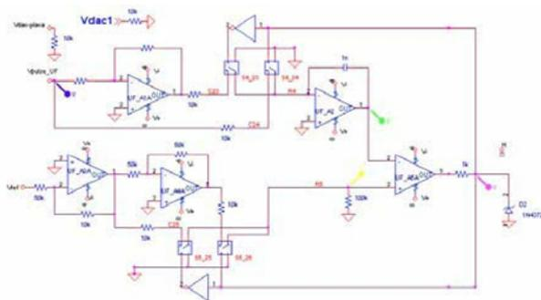
Figure 10. Voltage to frequency converter
