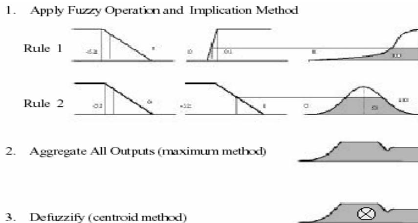
Figure 6 Graphical Inference and Defuzzification
