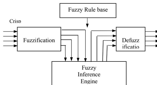
Figure 4. The fuzzy logic diagnostic system
