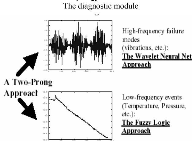
Figure 1 The two-prong approach of the diagnostic module
