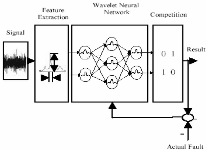
Figure 7 Classification using the wavelet neural network
