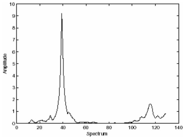
Spectrum domain for a defective bearing
