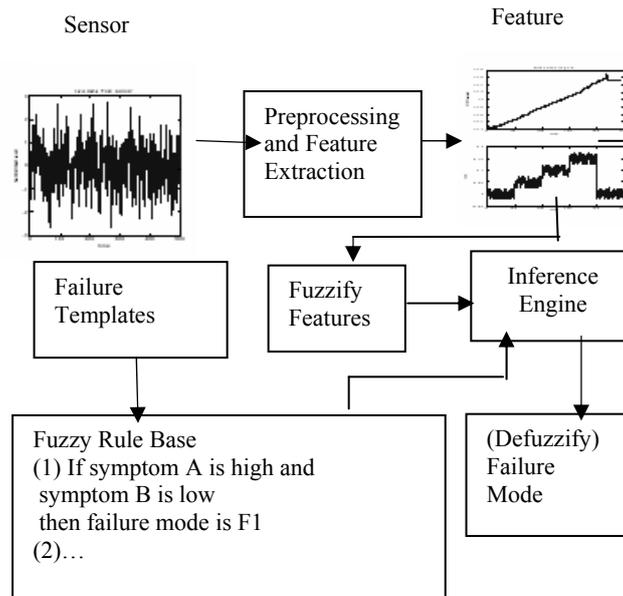
Figure 2. Fuzzy diagnostic system layout with feature extraction
